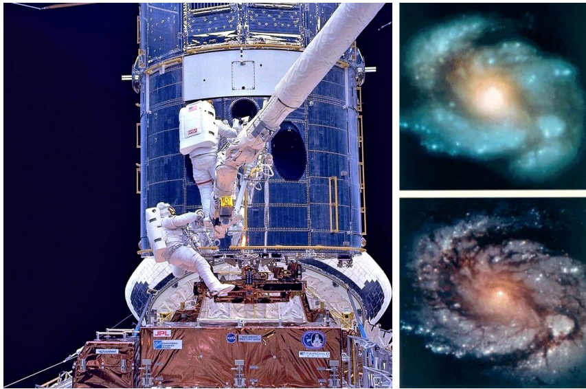
1 / The Hubble Space Telescope was placed into orbit with faulty optics in 1990. Its main mirror was supposed to have been nearly parabolic, since it is an astronomical telescope, meant for producing images of objects at infinity. However, contractor Perkin Elmer had delivered a faulty mirror, which produced aberrations. The large photo shows astronauts putting correcting mirrors in place in 1993. The two small photos show images produced by the telescope before and after the fix.
